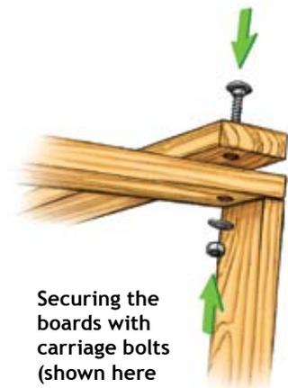
Securing the boards with carriage bolts (shown here without mesh on frame).
